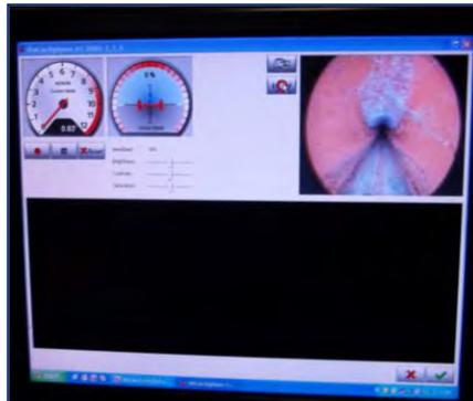
Double left click with mouse cursor on the calibration icon located in the upper right corner of the Digisewer screen. The calibration screen will then be displayed.
